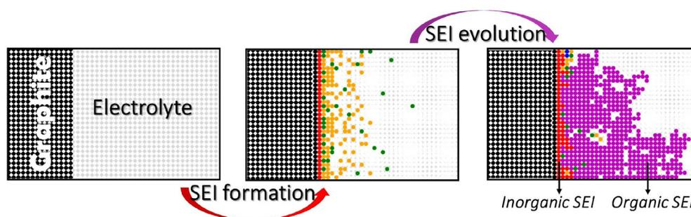
**Figure 1.** Schematic illustration of SEI formation and growth at the anode-electrolyte interface in LIBs.
